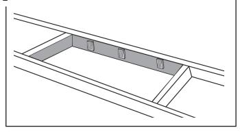
MAKE A ROUGH OPENING IN THE CEILING, AS SHOWN ABOVE. IF THE LADDER IS WIDER THAN YOUR JOIST CENTRES, YOU SHOULD CONSULT AN STRUCTURAL ENGINEER FOR ADVICE.
