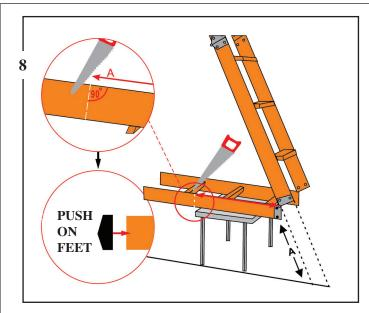
USING A HACKSAW, CUT LADDER TO THE CORRECT MEASUREMENT, FROM THE HINGE LINE, TO THE GROUND AND FIT PLASTIC FEET.
