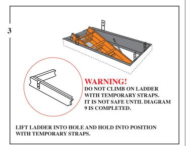
THERE ARE 4 TEMPORARY SUPPORT STRAPS SUPPLIED WITH THIS LADDER. WHEN YOU ARE SATISFIED WITH THE POSITION OF THE LADDER, BEND THE STRAPS OVER THE CEILING JOISTS AND SECURE WITH LARGE HEAD NAILS.
